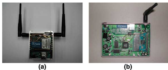
Fig. 1. Examples of mesh routers based on different embedded systems: (a) PowerPC and (b) Advanced Risc Machines (ARM).
